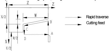
Fig. 14 Inner/outer cylindrical (taper) surface turning cycle Relationships between the data behind U, W, R and the tool path are as follows: (1)U<0, W<0, R<0 (2)U<0, W<0, R>0
