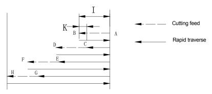
Fig. 22 G74 cycle- deep hole drilling cycle (R≠0)
