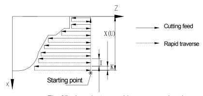
Fig. 25 Inner/outer roughing compound cycle
