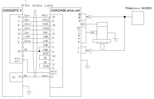
Connection layout between GSK928TE II CNC and GSK DA98 AC servo drive unit
