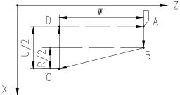
X from A to B is positive, so U>0; Z from B to C is negative, so W<0; X from C to B is negative, so R<0.
