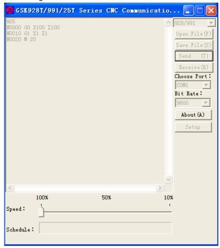
At the time, CNC automatically the sending state after it starts. If CNC does not start within 2 minutes, the communication program pops-up the prompt dialogue box: CNC does not start and is needed to recover.
