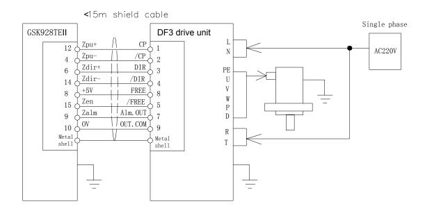
Connection layout between GSK928TE II CNC and GSK DF3:
