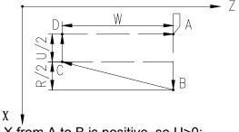
X from A to B is positive, so U>0; Z from B to C is negative, so W<0; X from C to B is positive, so R>0.
