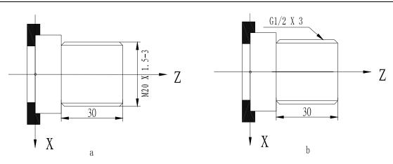
Fig. 35 Multiple threads cutting
