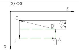
Diameter difference between starting point B and end point C is positive, so R>0
