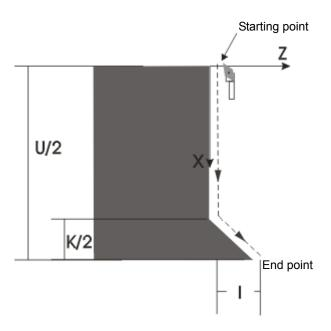
K sign decide the direction of the thread run-out; when K is omitted, there is no the thread run-out; when there is no I, I=K/2.
