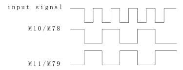
d) Pulse control mode: output sequence of M10, M11, M78, M79 controlled by pedal switch is as follows:
