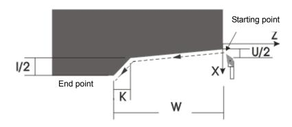
U sign decides the direction of the thread run-out; K sign is invalid; the machining cannot execute the rotary machining; when there is no I, I=2K.
