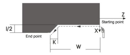
K sign decides the direction of the thread run-out; there is no the thread run-out when K is omitted; when there is no I, I=2K.
