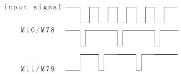
Note: The output duration of M10, M11, M78, M79 is defined by P15.
