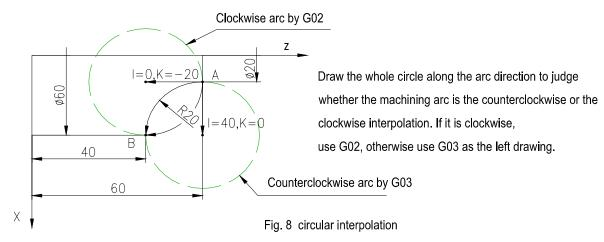
The feedrate of clockwise interpolation from A to B is 100 mm/min as Fig. 8: :
