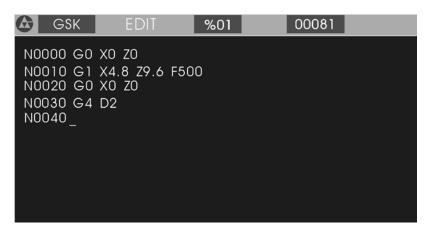
Fig. 8 automatically creating block number and inputting program content
