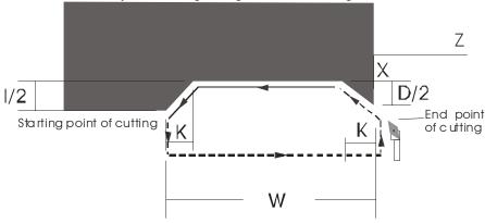
P is positive; K sign decodes the directions of the rotary machining and the thread run-out; K must not be omitted; when there is no I, I=2K.
