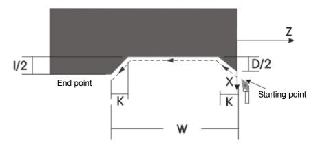
K sign decides the direction of the rotary machining and the thread run-out; K cannot be omitted; when there is no I, I=2K.
