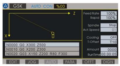
Fig. 19 Path of tool nose display in AUTO mode
