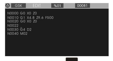
Fig 9. Generating a new block number after is pressed
