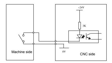
3.6.4 SP, ST signals use the normally open contact of mechanical contact switch; ESP with the normally-closed contact of self-lock mechanical contact switch.
