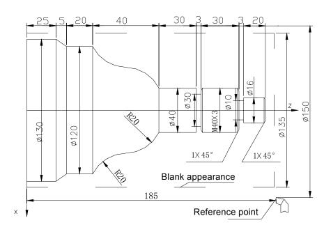
Fig. 36 Machining example
