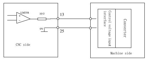
**I** The system is connected with the converter by the shield cable.
