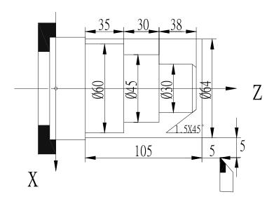
Fig. 33 Outer cylindrical surface machining
