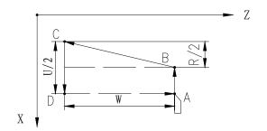
X from A to B is negative, so U<0; Z from B to C is negative, so W<0; X from C to B is positive, so R>0. (4)U<0, W<0, R>0
