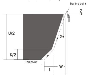
W sign decides the direction of thread run-out; K sign is invalid; the machining is rotary machine; when there is no I, I=K/2.
