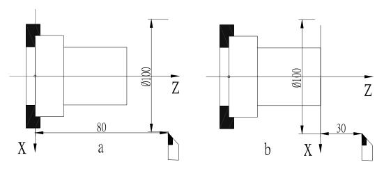
Fig. 12 G 50 creating a workpiece coordinate system
