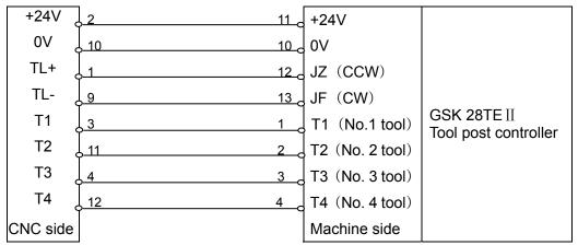
It is recommended that the tool post control line should be connected to CNC by the shield cable, and the shield and the shell of socket should be connected.
