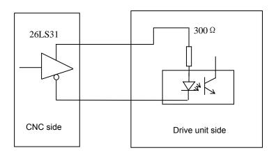
3.5.4 GSK928TE II CNC and compound stepper motor drive unit connection
