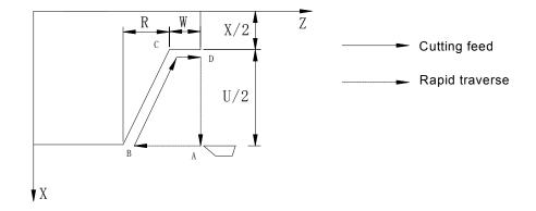
Fig. 18 G94 end face turning cycle
