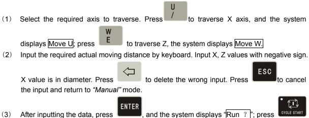
to traverse the selected axis according to the input distance and the direction.
