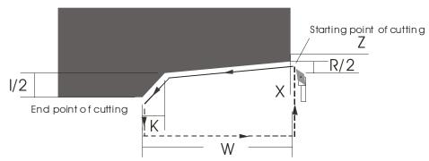
P is positive; R sign decides the direction of the thread run-out; K sign is invalid; there is no the rotary machining; when there is no I, I=K/2.
