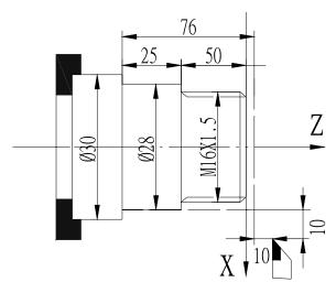
Fig. 34 Thread machining
