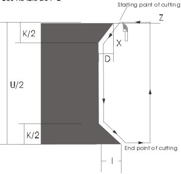
It is necessary to execute the cutting feed many times, at the moment, only rewrite X coordinate value of end point of cutting feed (or the increment value compared to the starting point). The coordinate position is still on the starting point when the thread cycle ends. Relationships between the sign of R, K and the tool path are as follows:
