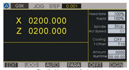
Fig. 12 Manual step feed mode
