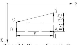
X from A to B is negative, so U<0; Z from B to C is negative, so W<0; X from C to B is negative, so R<0.
