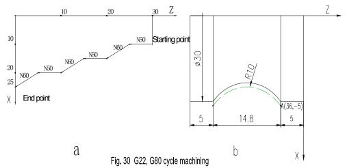
Machining the workpiece as Fig. 30a cycle programming with G22, G80 as follows:
