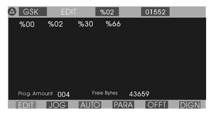
Fig. 3 Searching a part program catalog / creating, selecting and deleting part programs Most  $\%00 \sim \%99$  program names are displayed in each screen. When part programs in memory area are over 100, they are displayed by paging. Press to display the program number list of first page till the last page.
