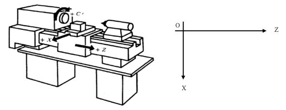
Fig. 1 X—Z plane rectangular coordinate system
