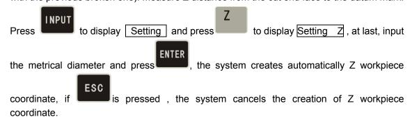
Clear out the previous system offset after the workpiece coordinate system has been created as the above-mentioned operation. If the workpiece coordinate system is not created, there is warp between the current X, Z coordinate values displayed and the actual tool position. Initialize the system before creating the workpiece coordinate system.
