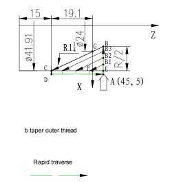
Fig. 17 G92 thread cutting cycle
