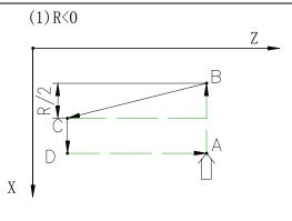
Diameter difference between starting point B and end point C is negative, so R<0
