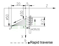
Fig. 15 Relationships between signs of U, W, R and tool path in G90
