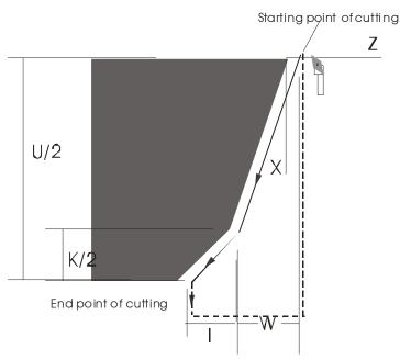
P is negative; R sign decides the direction of the thread run-out; K sign is invalid; there is no the rotary machining; when there is no I, I=K/2.
