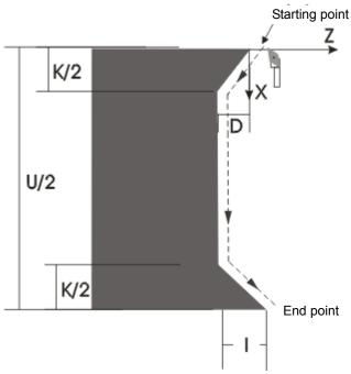
K sign decide the direction of the thread run-out; when K is omitted, there is no the thread run-out; when there is no I, I=K/2.
