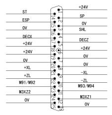
X3 Spindle encoder(male socket)
