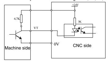
The valid level of VT is the LOW, i.e. the corresponding tool selection signal conducts with 0V when the tool selection signal is in-position.
